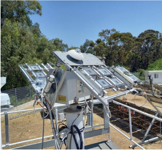
Figure 1: Perovskite mini-modules mounted outdoors on a tracker at the University of Cyprus site.
